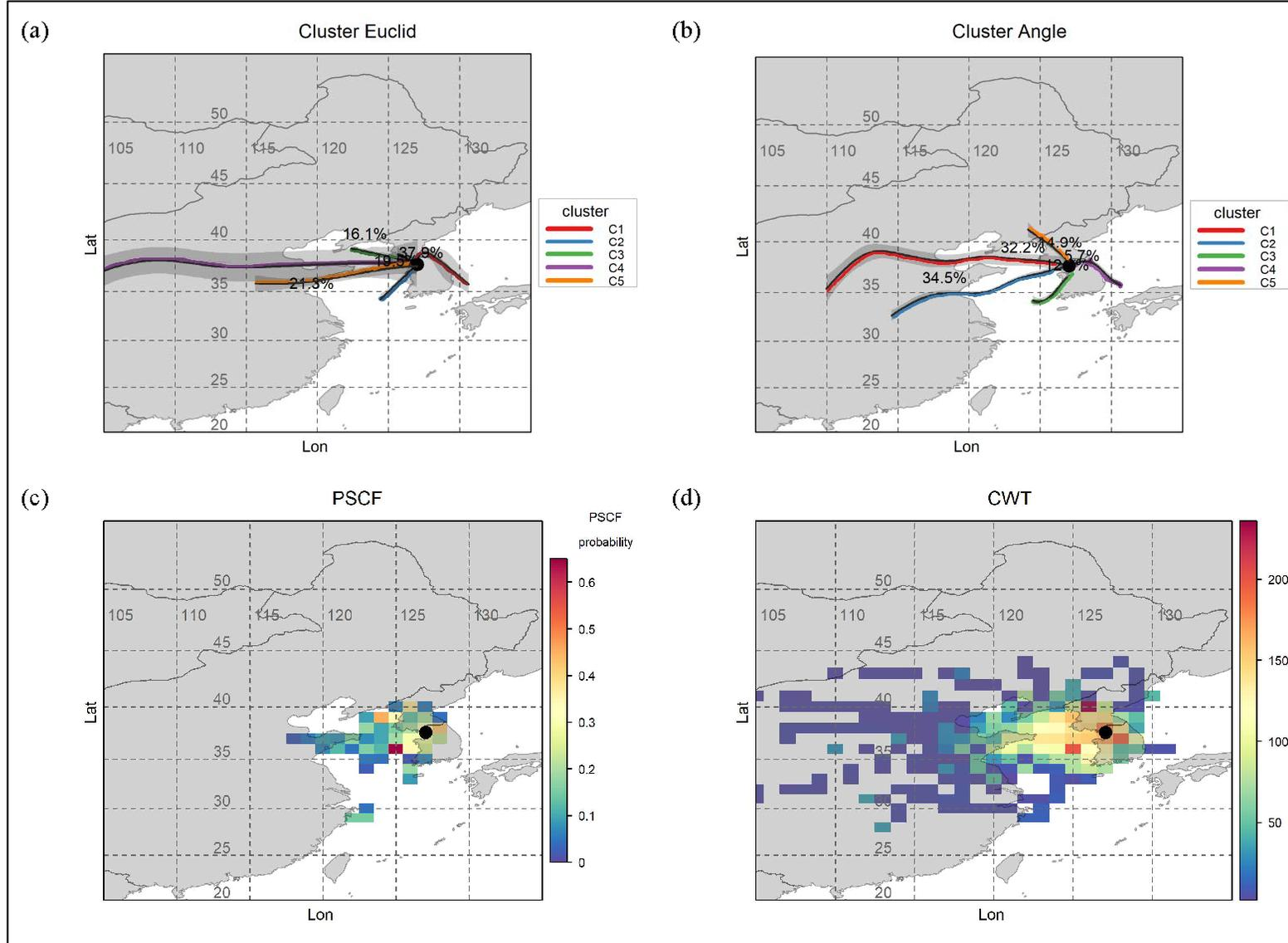
Figure 12: (a) Trajectories clustered by the Euclidian distance function, (b) trajectories clustered by the angle distance function, (c) the potential source contribution factor plot, and (d) the concentration-weighted trajectory plot
