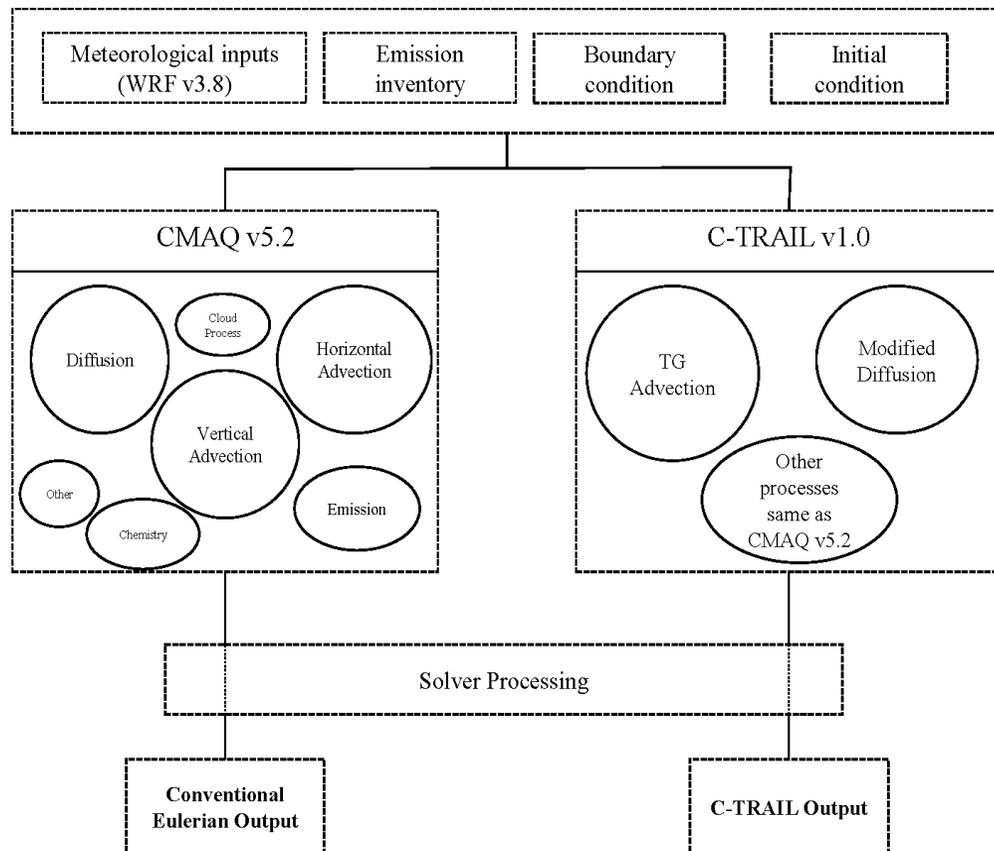
**Figure 1: Schematic of conventional CMAQ versus C-TRAIL**
