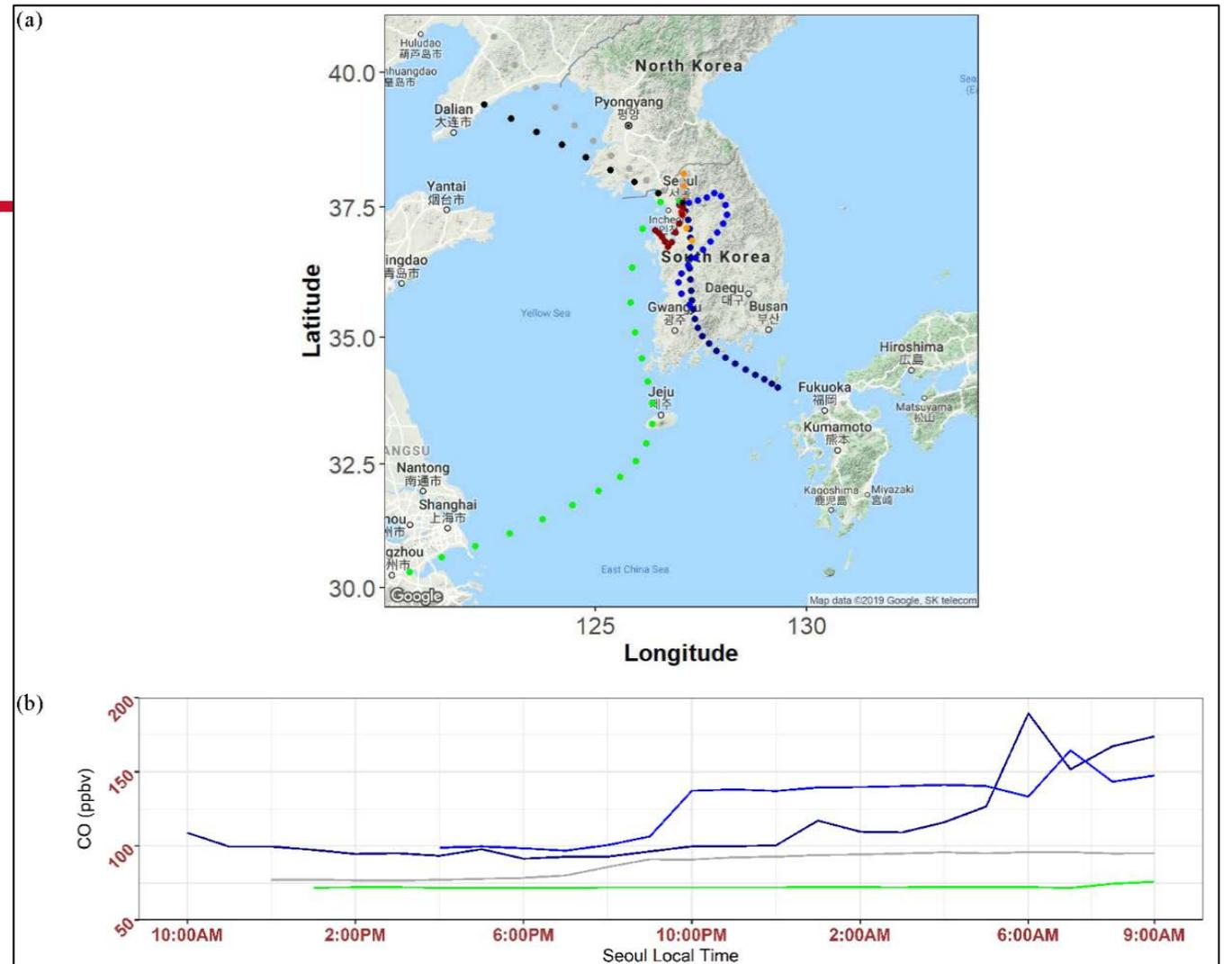
Figure 6: C-TRAIL output for June 4, 2016: (a) the trajectory of packets reaching Seoul at 9:00 AM local time (b) changes in the CO concentrations of four aged packets moving toward Seoul from source points
