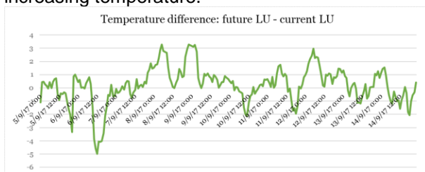
Fig. 5. Temperature (at 2m) difference between an urban cell classified as LCZ 1 (on a future scenario of urban growth) and LCZ 3 (current situation).
