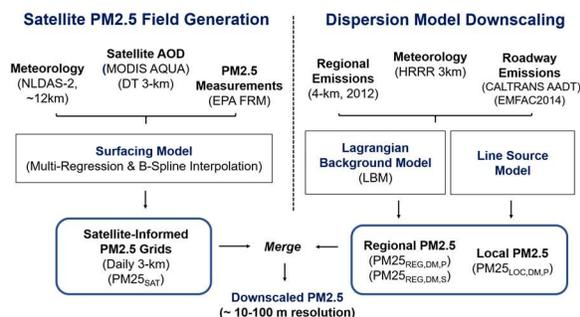
**Figure 1:** Components to construct regional PM<sub>2.5</sub> fields from MODIS Dark-Target 3-km satellite retrievals and downscale these to fine-scale using Lagrangian backwards and line-source dispersion models.
