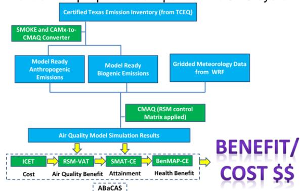
Fig.1. Schematic Diagram Showing Major Model Components Involved in ABaCAS-TX.
