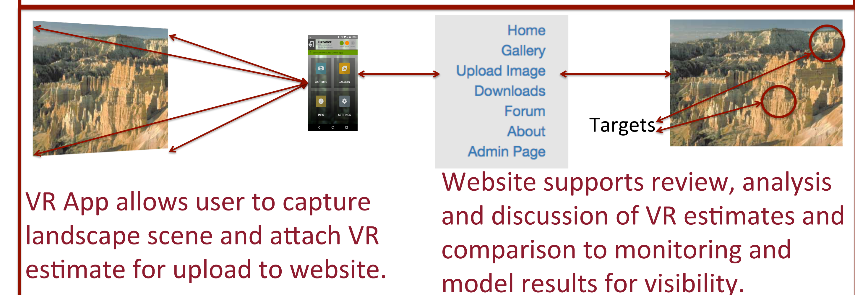
Figure 4. Visual Range Co-laboratory and Smart Phone App support exploring the value of Visual Range for estimating Air Quality, offering the possibility of using direct human observations of visibility to estimate air quality (PM2.5 or Air Quality Index). A smart phone (Android) app has been developed for capturing landscape scenes photographically and uploading these to a web site.
