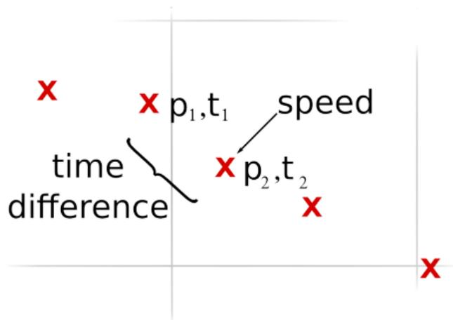
$$E(v, p_2, t_2) = \left( \frac{\text{speed}}{\text{speed}_{\max}} \right)^3 MCR_{\max} \Delta t EF + E_{\text{aux}}$$
