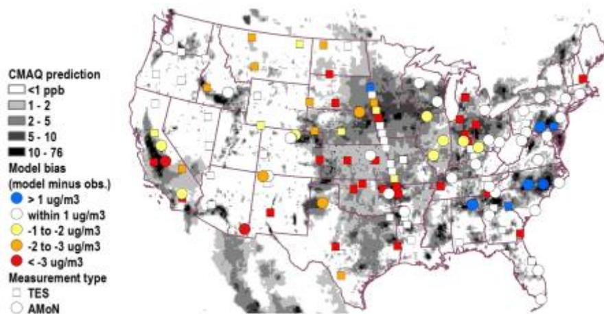
Figure 5. Spatial variation in model prediction error based on AMoN measurements and TES retrievals of surface concentrations over a background of model predictions.
