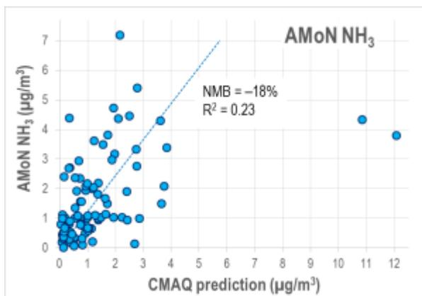
Figure 1. Ground level NH<sub>3</sub> measurements (AMoN) compared with model predictions.
