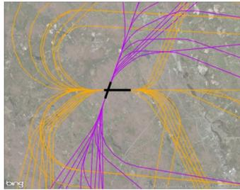
A hypothetical example of an airport with planned arrival and departure flight paths. These planned flight paths are described in two dimensions from which AEDT will calculate the arrival and departure altitudes and speeds based on specific airplane characteristics and aircraft control procedures.
