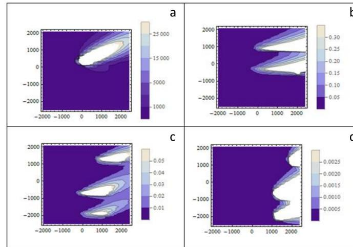
Figure 2: The distribution of PM emissions at ATL in units of  $\mu\text{g}/\text{m}^3$ . In alphabetical order: the emissions from engines running at the idle, takeoff, landing, and approach power settings.
