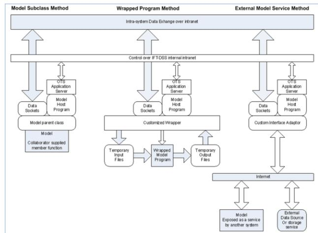
Fig. 3. IFT-DSS model integration methods
