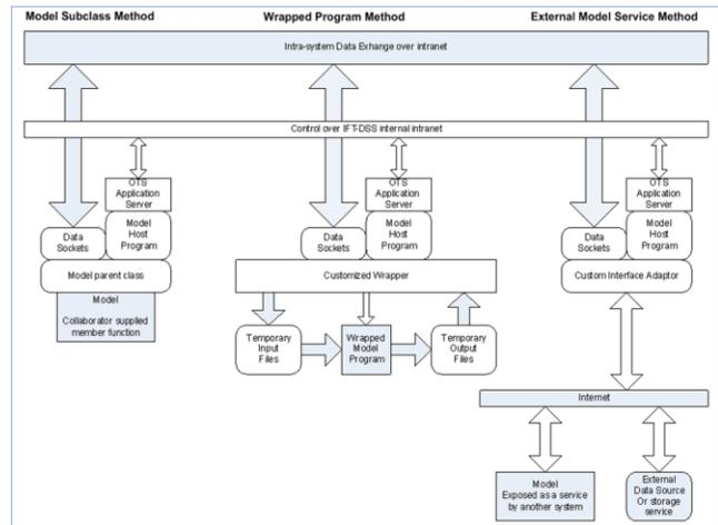
Fig. 3. IFT-DSS model integration methods
