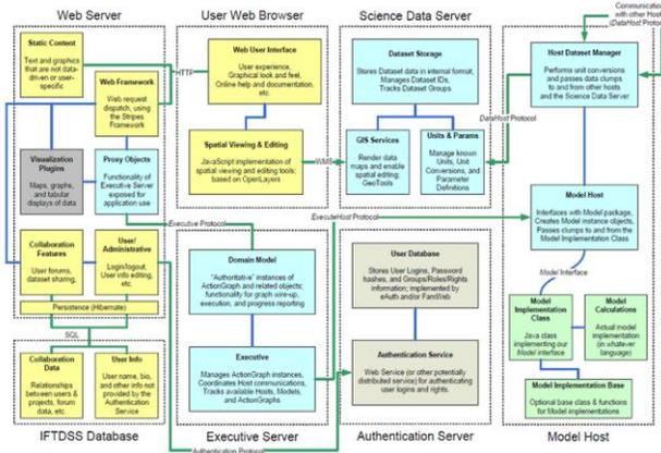
Fig. 4. IFT-DSS topology and the communication mechanisms.
