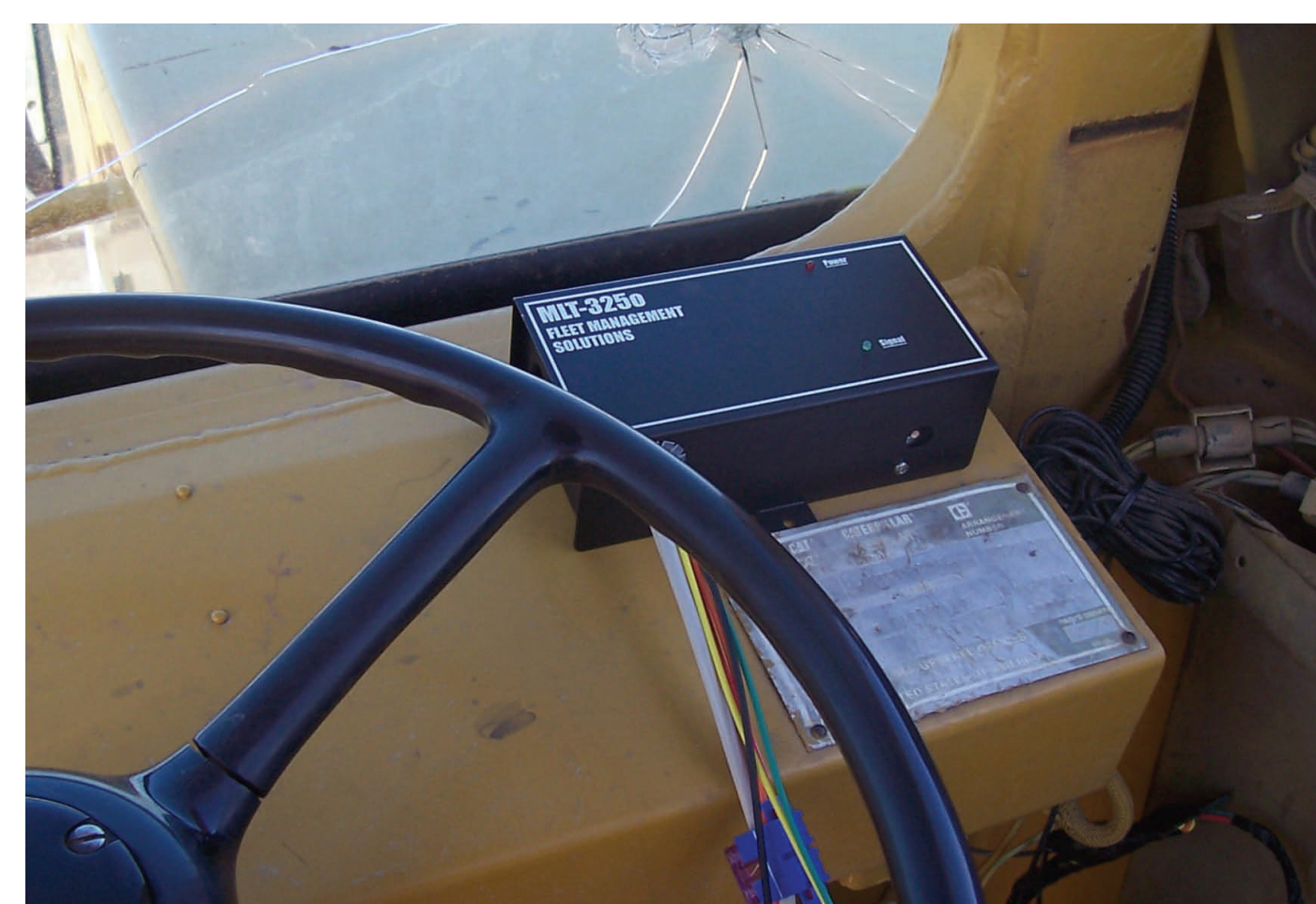
A GPS unit mounted in the cab of a John Deere 615C Scraper owned by Bison Construction Co.
