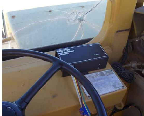
Fig. 2. GPS unit mounted in the cab of a John Deere 615C scraper.
