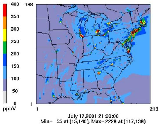
**Fig. 4.** CMAQ layer 1 12km grid modeled CO concentrations on July 17<sup>th</sup>, 2001 at 2100 GMT
