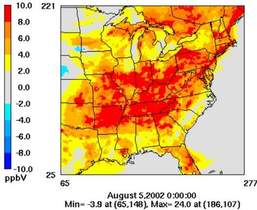
**Fig. 14.** 8-hour average ozone difference between CMAQ with RADM dry and M3Dry (RADM – M3Dry) on August 5<sup>th</sup>, 2002. Positive values are ozone increases due to RADM dry deposition.
