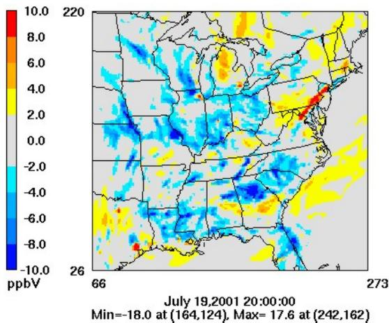
**Fig. 8.** One hour average ozone difference between CAMx run with O'Brien and “CMAQ like” Kv’s (CMAQ-like – O'Brien) on July 19<sup>th</sup>, 2001 at 20Z. Negative values are ozone reductions due to “CMAQ like” Kv’s.
