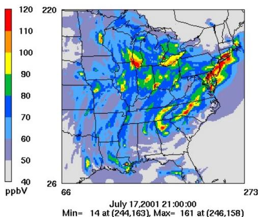
Fig. 1. CAMx 12km grid modeled ozone concentrations on July 17<sup>th</sup>, 2001 at 2100 GMT.
