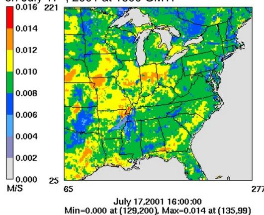
**Fig. 10.** CMAQ 12km grid deposition velocity (Vd) for CO (M3Dry) on July 17<sup>th</sup>, 2001 at 1600 GMT.
