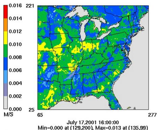
**Fig. 12.** CMAQ 12km grid deposition velocity (Vd) for O<sub>3</sub> (M3Dry) on July 17<sup>th</sup>, 2001 at 1600 GMT.
