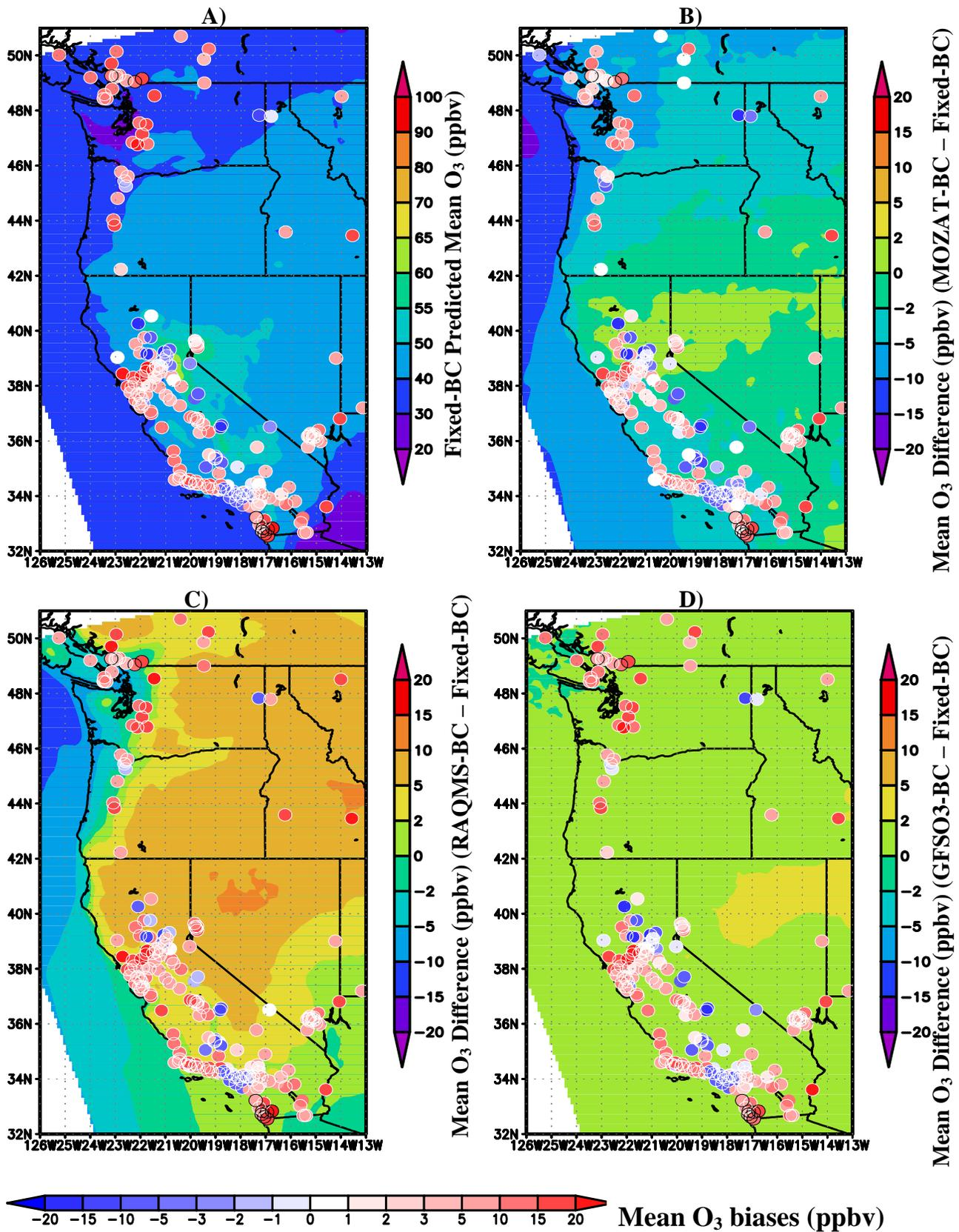
Figure 7, Mean surface O<sub>3</sub> prediction (plot A for Fixed-BC), mean O<sub>3</sub> prediction differences (B for MOZAR-BC, C for RAQMS-BC, D for GFS O<sub>3</sub> BC) and their mean biases from AIRNOW observations during Aug 1 to 5, 2006.
