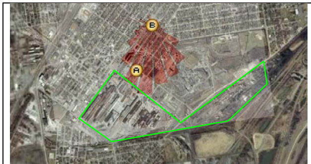
Figure 5. Wind analysis showing predominate wind directions when PM_{2.5} concentrations at the Granite City monitor (location B) exceed the regional background PM_{2.5} levels and outline of U.S. Steel Granite City Works facility (Source: Turner and Garlock, 2007).
