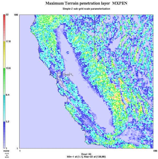
Figure 4: Maximum terrain penetration layer for the 4 KM *MM5* grid, using the Simple-Z sub-grid scale terrain parameterization. The maximum of layer 22 corresponds to an elevation of approximately 1000 meters.
