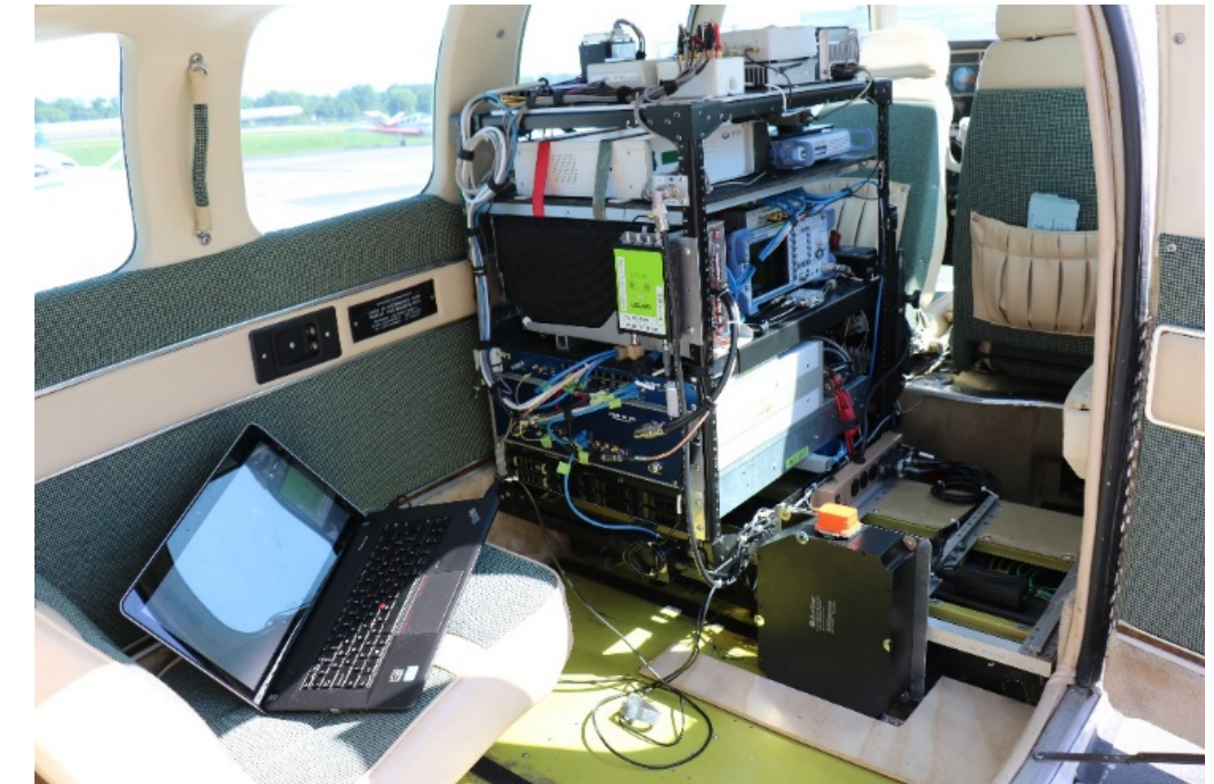
Figure 5: Customized SWIR spectrometer used during flight experiment (left), configuration of spectrometer inside aircraft (right)
