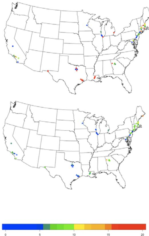
Fig 1. Observed (top) and modeled (bottom) TNMOC:NO<sub>2</sub> averaged over all hours where observed O<sub>3</sub> concentrations are ≥ 70 ppb (Triangle indicates N < 10, circle indicates N ≥ 10).
